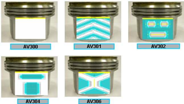
Figure 2. Skirt profile configuration of test pistons
